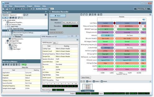
APx500 Measurement Software metadata recorder tracking metadata changes during an HDMI hotplug event.
